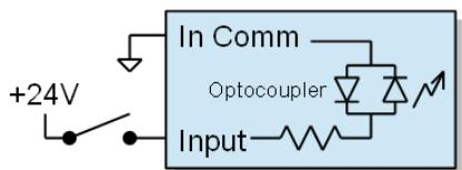
EStop behaves like an input and must be active to permit motion.
