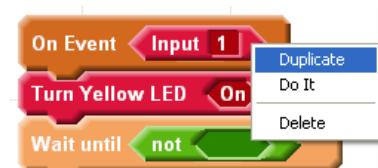
**Step 13)** Drag the duplicate diamond into the "Not" block diamond field. Click on the "IO" Category, drag another "Turn Yellow LED" block onto the list, left click the diamond field and select "Off".
