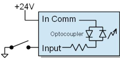
**Step 2 for sourcing)** If you have sourcing inputs then wire In Comm to 24 volts minus and your sensor to input 1
